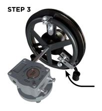
Put a washer (if included) on a bolt, pass the bolt through one of the two remaining slots in the chainwheel from the front. Pass through both sides of the U-Strap and fasten loosely with a lock washer (if included) and nut.
