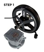
Pass a slotted bolt through the top slot of the chainwheel and pass the bolt through the long L strap. Hang the chainwheel on the valve hand wheel with the long L strap on the top (12 o'clock).
