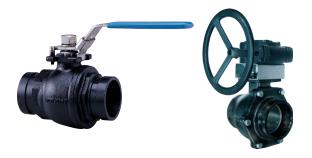
The Model SJ-500L is a ductile iron, grooved-end, two-piece, regular port ball valve designed and tested in conformance with MSS SP-110 and SP-72. The lever handle is equipped with tamper resistant locking holes. The SJ-500L is comprised of a ductile iron body and end cap, virgin TFE seats and chrome-plated carbon steel trim. Also available with stainless steel trim as an option.
